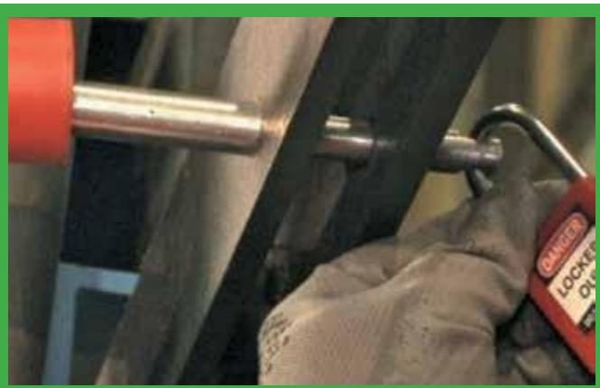
Mechanical Isolation: protecting a sliding door
