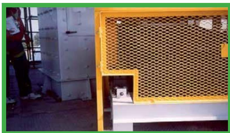
*Remote greasing to prevent the need to remove the machine guard.*
