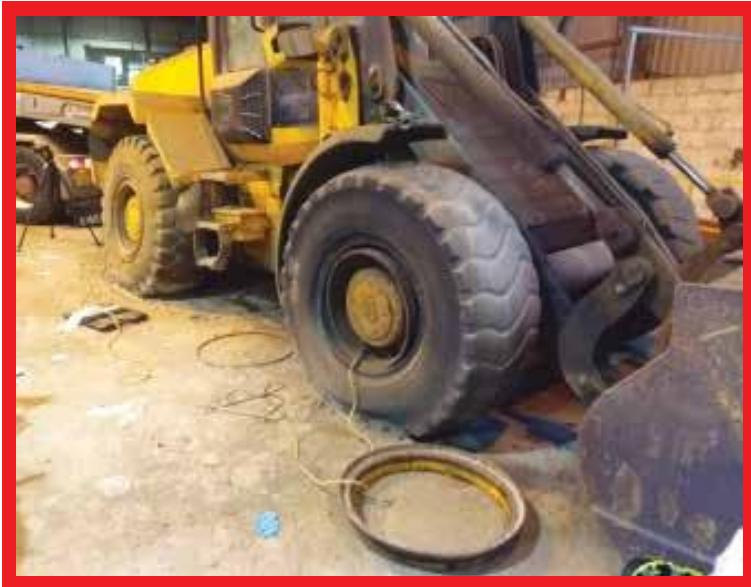
*While inflating the front offside tyre of a front end loader (which was being collected from a site by a third party), the tyre mechanism ruptured and the sealing ring was ejected and struck the operator. He died of his injuries. The airline used was connected to the compressor of the truck (of the deceased) and did not have a gauge or regulator fitted.*
