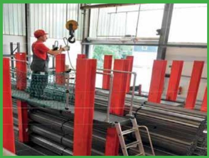
*Safe access for attaching lifting hooks.*
