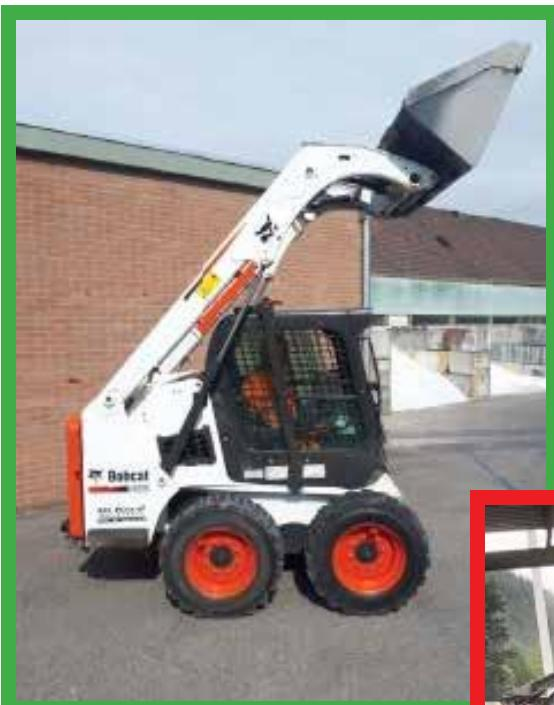
*2018: 2 employees died when the arms of the bobcat unit they were working on came down and crushed them while they were carrying out a repair – the safety lock on the machine had not been engaged.*
